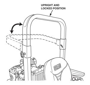
Figure 2-1. Foldable Roll-Over Protection System
